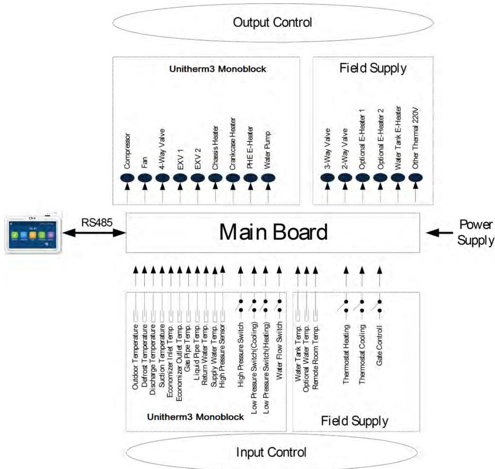
1. The outdoor temperature is detected by the sensor installed at fins of the finned heat exchanger, which is mainly used to control the initialization steps of the fan and the electrostatic expansion valve and also limit the maximum running frequency of the compressor. When this sensor fails, the main board will detect it and deliver this error message to the controller and then the unit will fail to start up or shut down.
