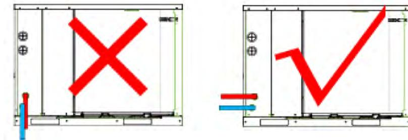
It is recommended to connect water pipe in horizontal direction. Do Not connect water pipe in vertical direction.
