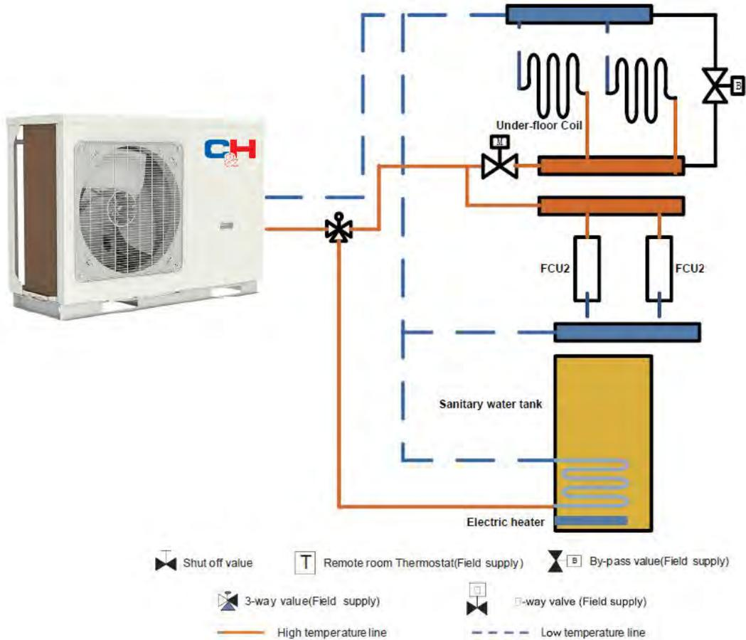
Two-way valve is very important to prevent dew condensation on the floor and radiator while cooling mode.
