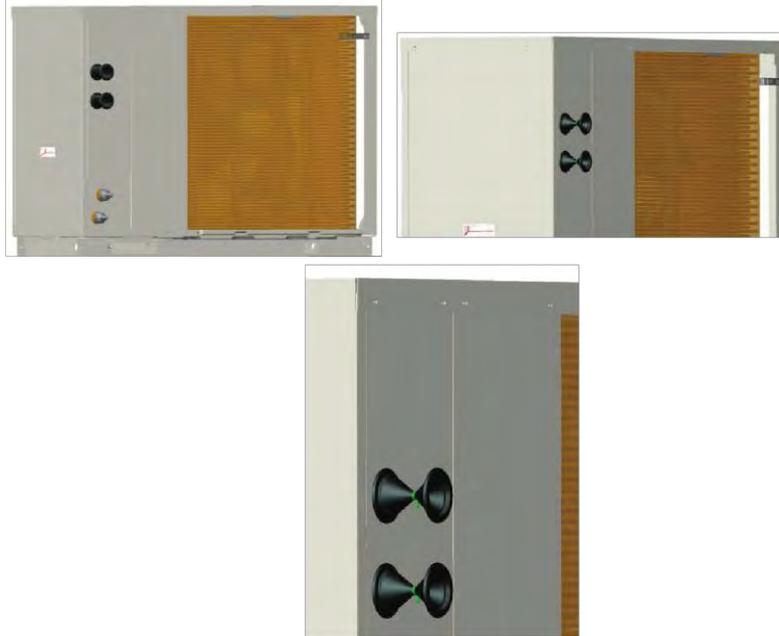
1. Take away the original rubber rings; replace the long tail rubber rings of accessory;
